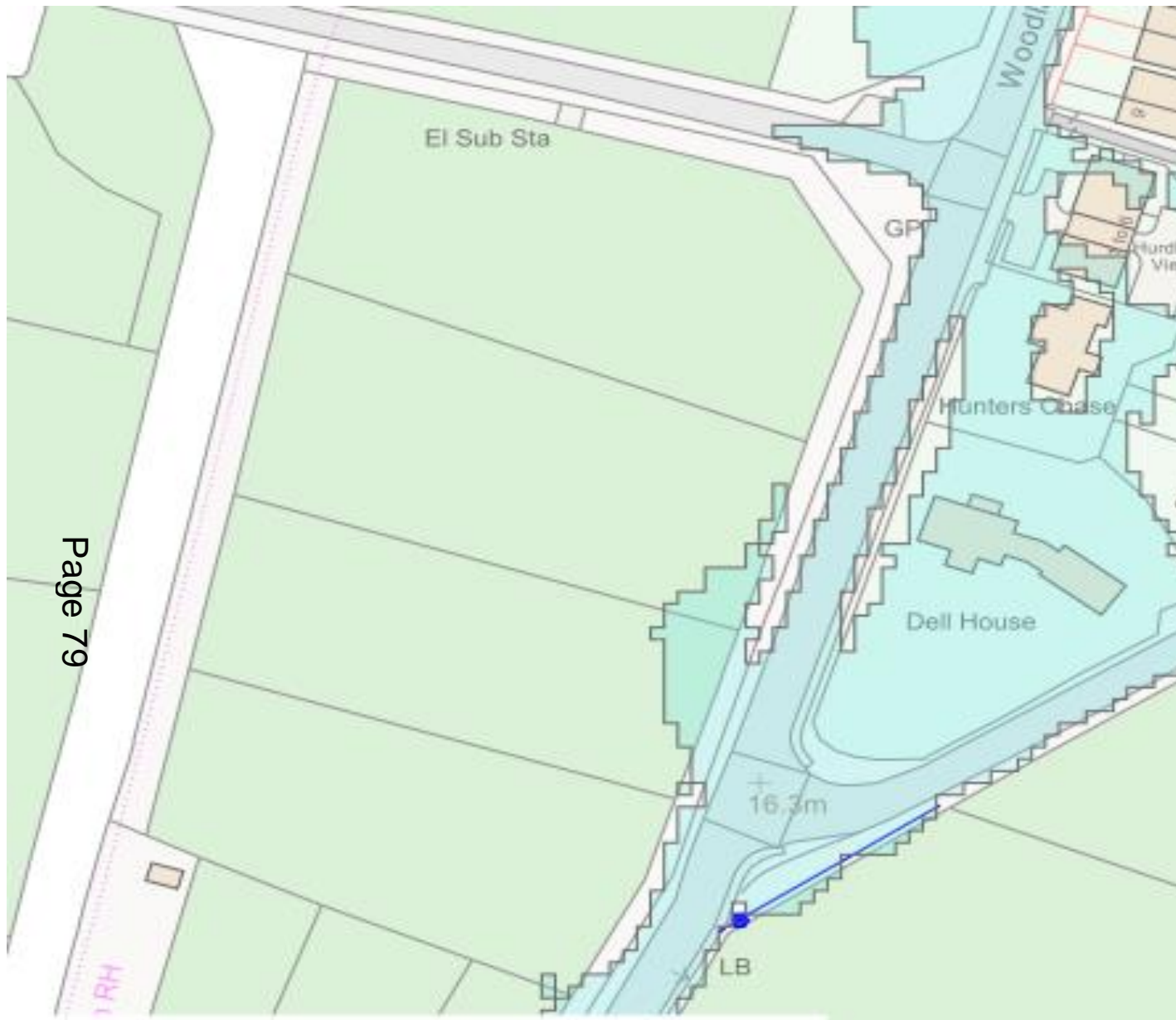
Extent of 1:1000 Year Surface Water Flooding in light blue with dark blue line as watercourse along Wandleys Lane and blue dot as position of culvert
